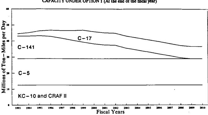
FIGURE 3. ESTIMATED CONTRIBUTION OF EACH TYPE OF AIRCRAFT TO AIRLIFT CAPACITY UNDER OPTION 1 (At the end of the fiscal year)
