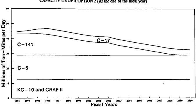
FIGURE 4. ESTIMATED CONTRIBUTION OF EACH TYPE OF AIRCRAFT TO AIRLIFT CAPACITY UNDER OPTION 2 (At the end of the fiscal year)
